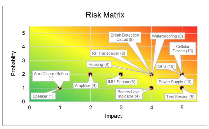
Fig. 7. Risk Matrix showing the Impact of component failure vs. the Probability of occurrence on a scale of 1 (low) to 5 (high). [11]
