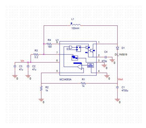
Fig. 11. Power Supply Schematic [15]
