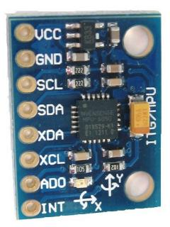
Fig. 3. InventSense MPU-6050 [9]
