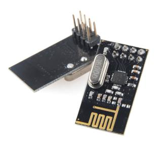
Fig. 5. A 2.4 GHz RF Transceiver [10]
