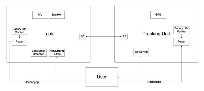
Fig. 10. Block Diagram of comBATS
